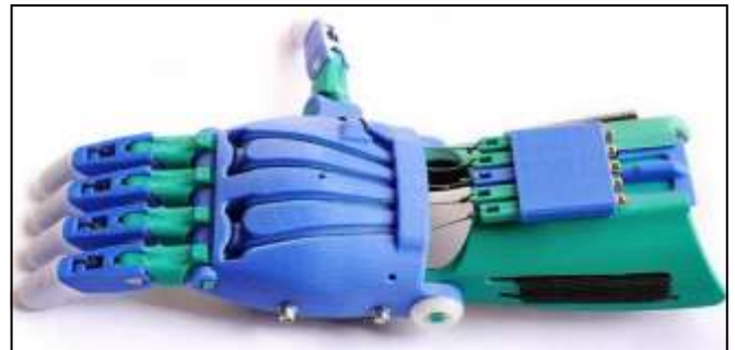
The prosthetic hands will be 3D printed using recycled plastic from shampoo and conditioner bottles.
